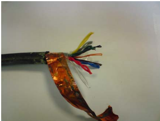
Fig 9. Rediffusion trunk distribution cable
